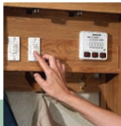
Interior Command Center® that controls generator and slideout functions
