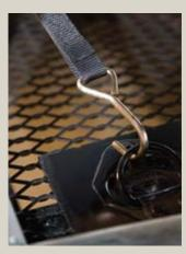
Six D-rings on the front deck safely secure your bikes or ATV.
