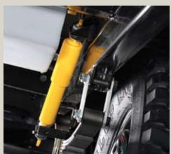
For smoother trips through rugged terrain, Baja camping trailers are built with 13 inches of ground clearance plus leaf springs and shock absorbers.
