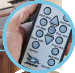
KEY FOB REMOTE FOR SLIDEOUTS, PATIO AWNING/LIGHT, POWER JACKS
