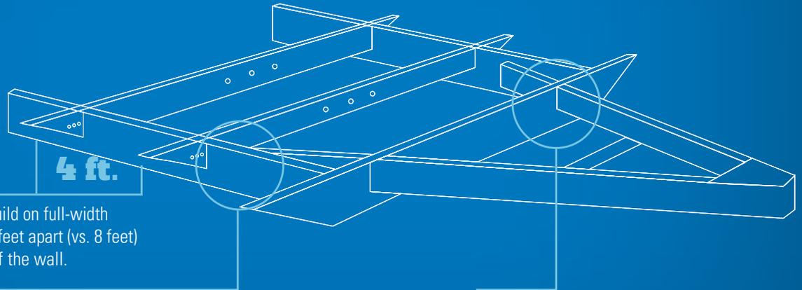
**Full-width outriggers:** We build on full-width outriggers that are spaced 4-6 feet apart (vs. 8 feet) to better support the weight of the wall.
